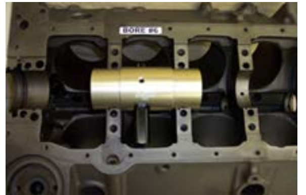
Fig #12 To clear for #6 rod keep the flange closest to the pointer against main saddle #4.
