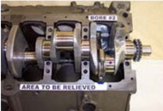
Fig #1 To set the Stroker Mimic we recommend creating a relief in the block for rod #2 at the pan rail area, using your normal process( crank, rod, piston and bearings).
