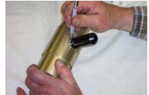
Fig #6 Once satisfied with the setting, scribe a line on the pointer opposite the set screw, utilizing the flat provided in the arbor or measure and record so it is possible to return to that setting for future use. Scribe or measure a different position for each new rod and stroke combination.
