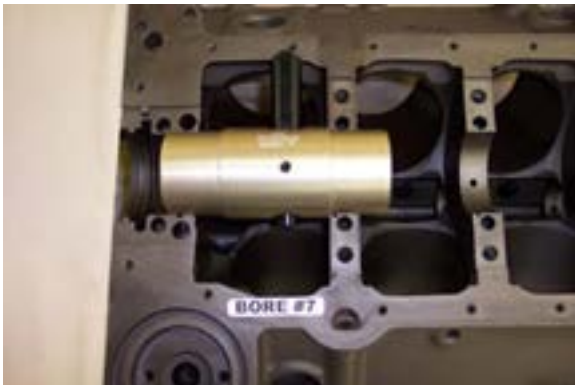
Fig #13 To clear for #7 rod keep the flange closest to the pointer against main saddle #4.
