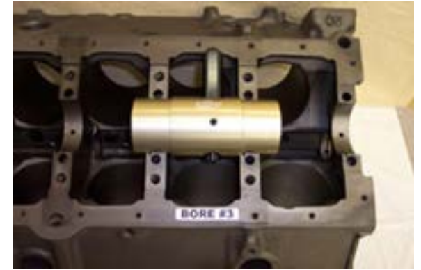
Fig #9 To clear for #3 rod keep the flange closest to the pointer against main saddle #2.
