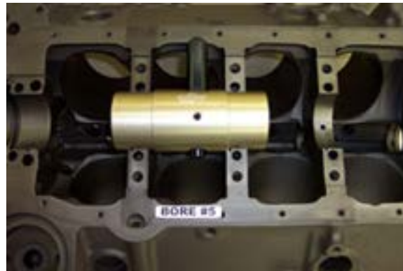
Fig #11 To clear for #5 rod keep the flange closest to the pointer against main saddle #3.
