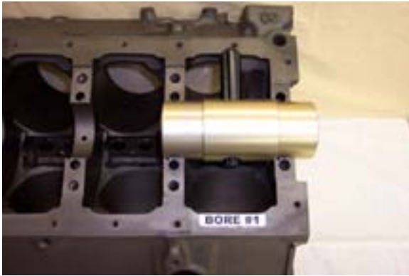
Fig #7 To clear for #1 rod keep the flange farthest from the pointer against main saddle #1.
