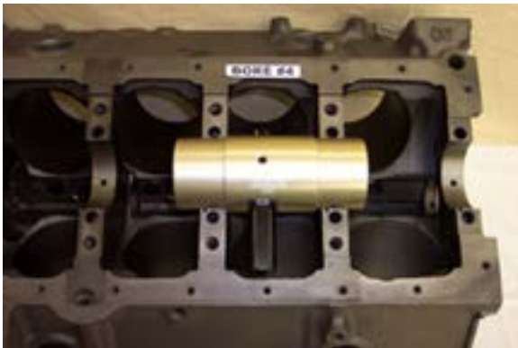
Fig #10 To clear for #4 rod keep the flange closest to the pointer against main saddle #3.
