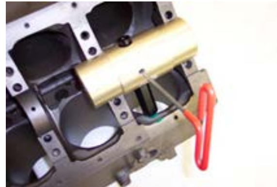
Fig #5 Lock the pointer in position with the set screw and check the clearance again.
