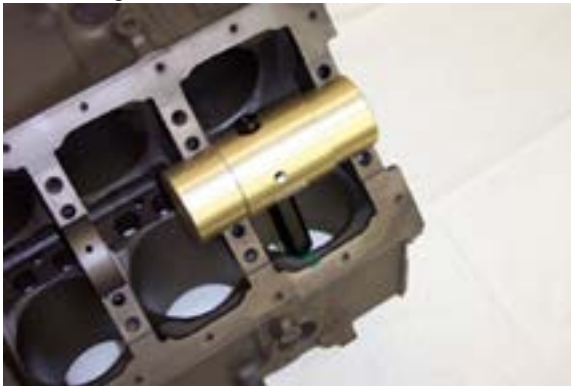
Fig #4 Rotate the arbor and adjust the pointer in or out until the tapered end of the pointer passes freely thru the relief with a minimum of clearance.
